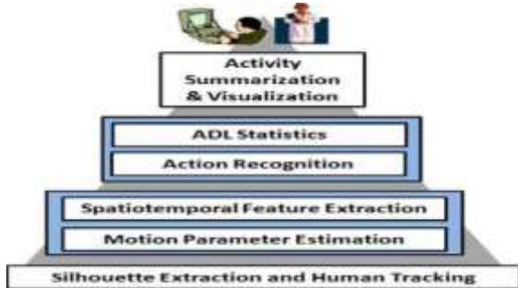
Fig 1. Overview of the proposed framework for automated activity analysis, summarization and visualization
